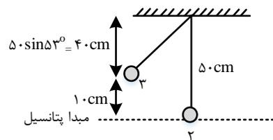
$$mgh_1 = \frac{1}{2}mV_2^2 \xrightarrow{g=10 \frac{m}{s^2}, h_1=0.2m} 10 \times 0.2 = \frac{1}{2} \times V_2^2 \rightarrow V_2^2 = 4 \rightarrow V_2 = 2 \frac{m}{s}$$
